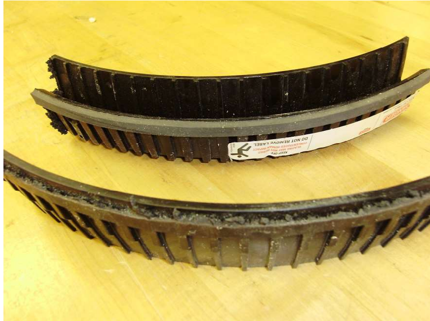
Photo No. 1 Thick material (top specimen) Thin material (bottom specimen) Polypropylene Support-Test materials for: ASTM D 1929-01 ASTM D 2843-04 ASTM D 635-06
